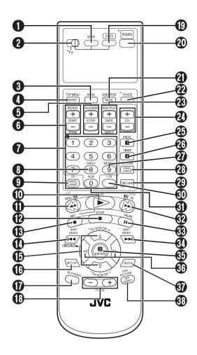
Buttons with a small dot on the left side of the name (POWER (७/١), TV/VCR, TV/VCR CH +/-, TV VOL+/-, MUTE) can also be used to operate a JVC's TV after setting the TV/VCR/DVD switch to the left.
